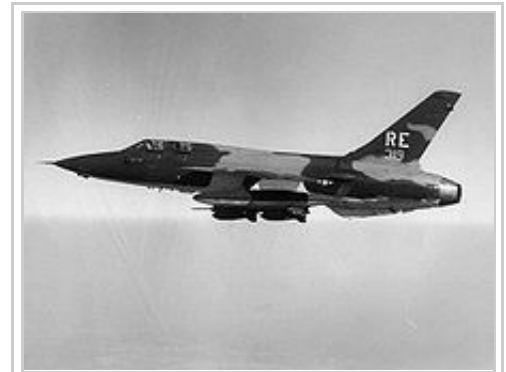
Republic F-105F-1-RE Thunderchief Serial 63-8319 from the 44th TFS Later, this aircraft was reconfigured to the F-105G "Wild Weasel" configuration.
